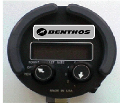
LCD displays range in meters, directional bearing, transmit and receive functions, channel selection, and low battery indicator.
